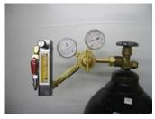
After connecting the BK assembly to the compressed breathing air source to be analyzed, the breathing air is passed through each detector tube at a specific pressure, flow rate and time interval. Each detector tube is made with high purity reagents that absorb and react with the target component. The reaction causes a colorimetric stain whose length is proportional to the component's concentration. The actual concentration is read directly from the measurement scale printed on the detector tube.
